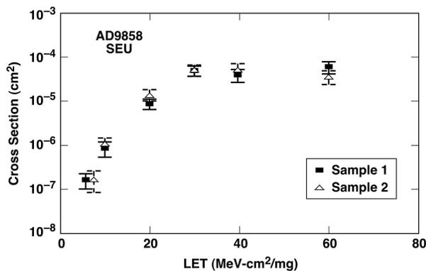
Fig. 6. Comparison of data obtained for two samples at room temperature for AD9858. Measurements were performed at the TAM.
