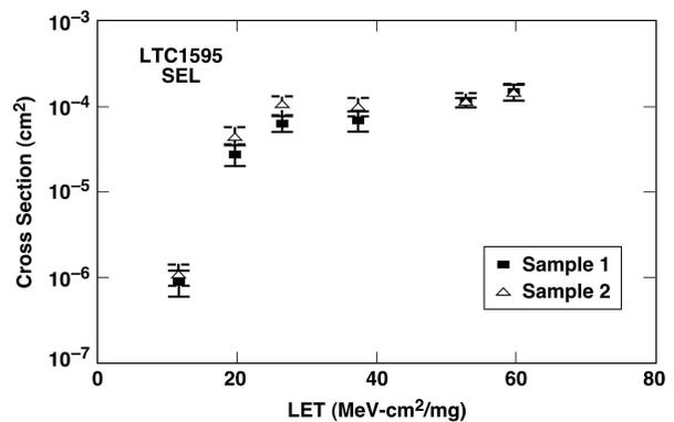
Fig. 4. Comparison of data obtained for two samples at room temperature for LTC1595. Measurements were performed at the BNL.
