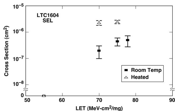
Fig. 1. Comparison of data obtained at room temperature with the heated measurement for LTC1604. Measurements were performed at the TAM.
