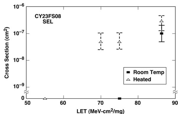
Fig. 8. Comparison of data obtained at room temperature with the heated measurement for CY23FS08. Measurements were performed at the TAM.
