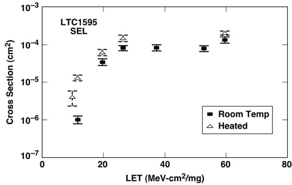
Fig. 5. Comparison of data obtained at room temperature with the heated measurement for LTC1595.
