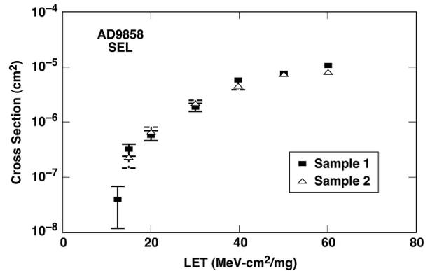
Fig. 7. Comparison of data obtained for two samples at room temperature for AD9858. Measurements were performed at the TAM.
