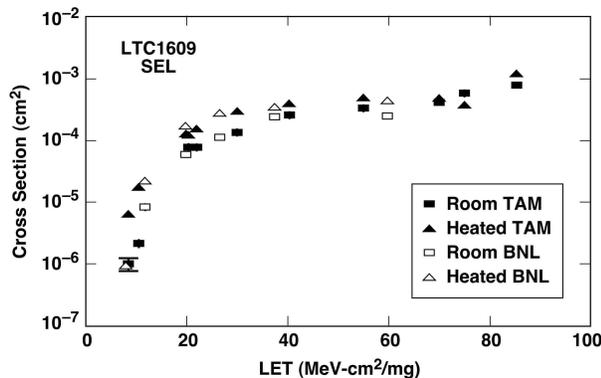
Fig. 3. Comparison of data obtained at TAM facility and BNL facility for both room temperature and heated measurement for LTC1609.
