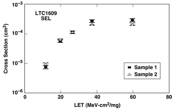
Fig. 2. Comparison of data obtained for two samples at room temperature for LTC1609. Measurements were performed at the BNL.
