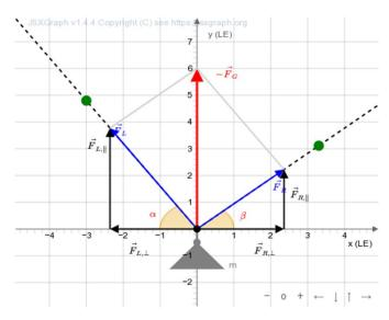
Fig. 3: Interactive picture in which the given force  $-F \stackrel{\cdot}{\_}G$  for any angle  $\alpha$  and  $\beta$  can be decomposed along the two dashed lines by moving the two green dots
