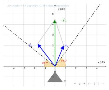
Fig. 1: Decomposition of the force -F <sup>^</sup>\_G into the two forces F <sup>^</sup>\_L and F <sup>^</sup>\_R (blue vectors) along the dashed lines.
