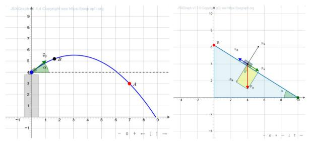
Fig. 4: Determination of the maximal potential and kinetic energy on a trajectory of a projectile via movement of dots A and B (left panel). Determination of the minimal angle of the plane to overcome the friction force via adjustment of the dot S (right panel
