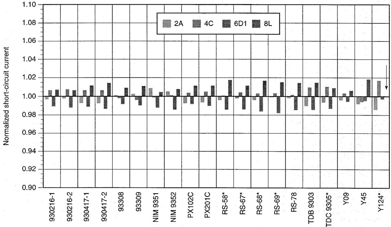
Fig. 2. Normalized reference cell calibration results for the WPVS sample set following removal of secondary calibrations (1, 9, and 10) and laboratories with 50% or more data points exceeding  $1.0 \pm 0.02$  (3, 5, and 7). The  $2\sigma$  standard deviation is 1.9%. The point marked with a vertical arrow was removed as an outlier. Cells indicated with a (\*) had defects that may affect the calibration uncertainty.
