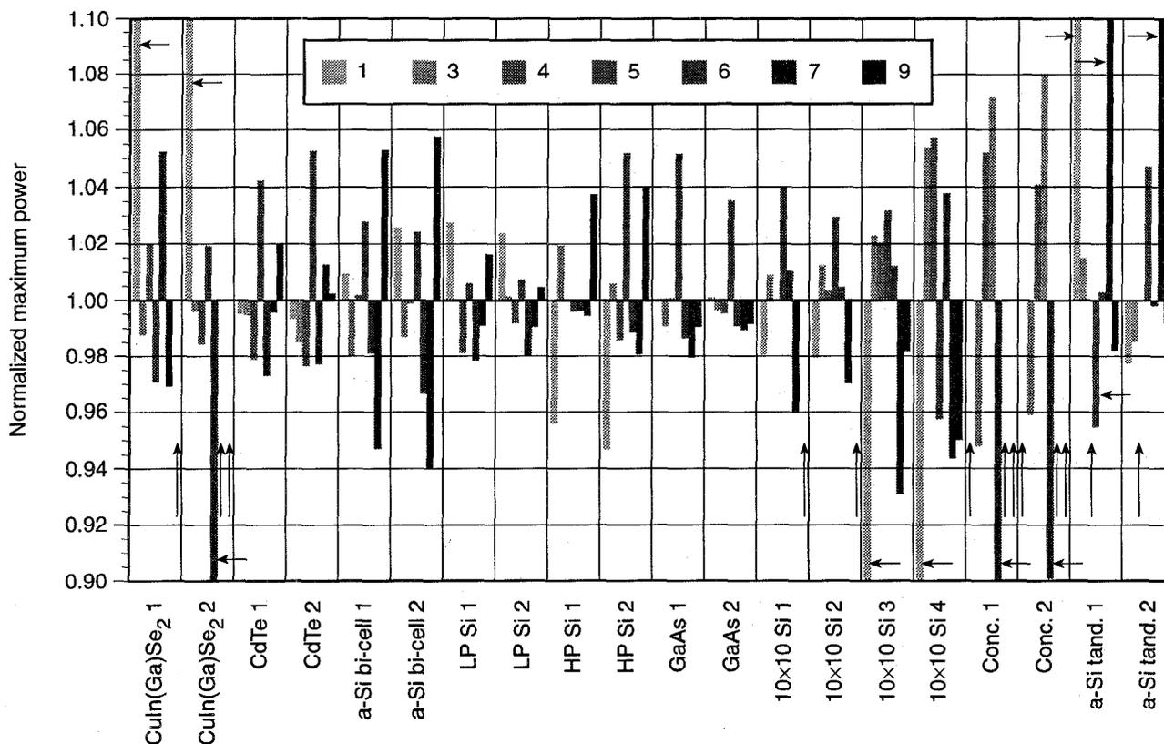
Fig. 3. Normalized maximum-power results for the NT series sample set. The  $2\sigma$  standard deviation is 5.7%. The vertical arrows mark missing data points, and the horizontal arrows indicate data points that exceeded  $1.0 \pm 0.08$ . All but one of these points exceeded  $1.0 \pm 0.1$  and were clipped to the plot edges. These outliers were not used to calculate the overall standard deviation.
