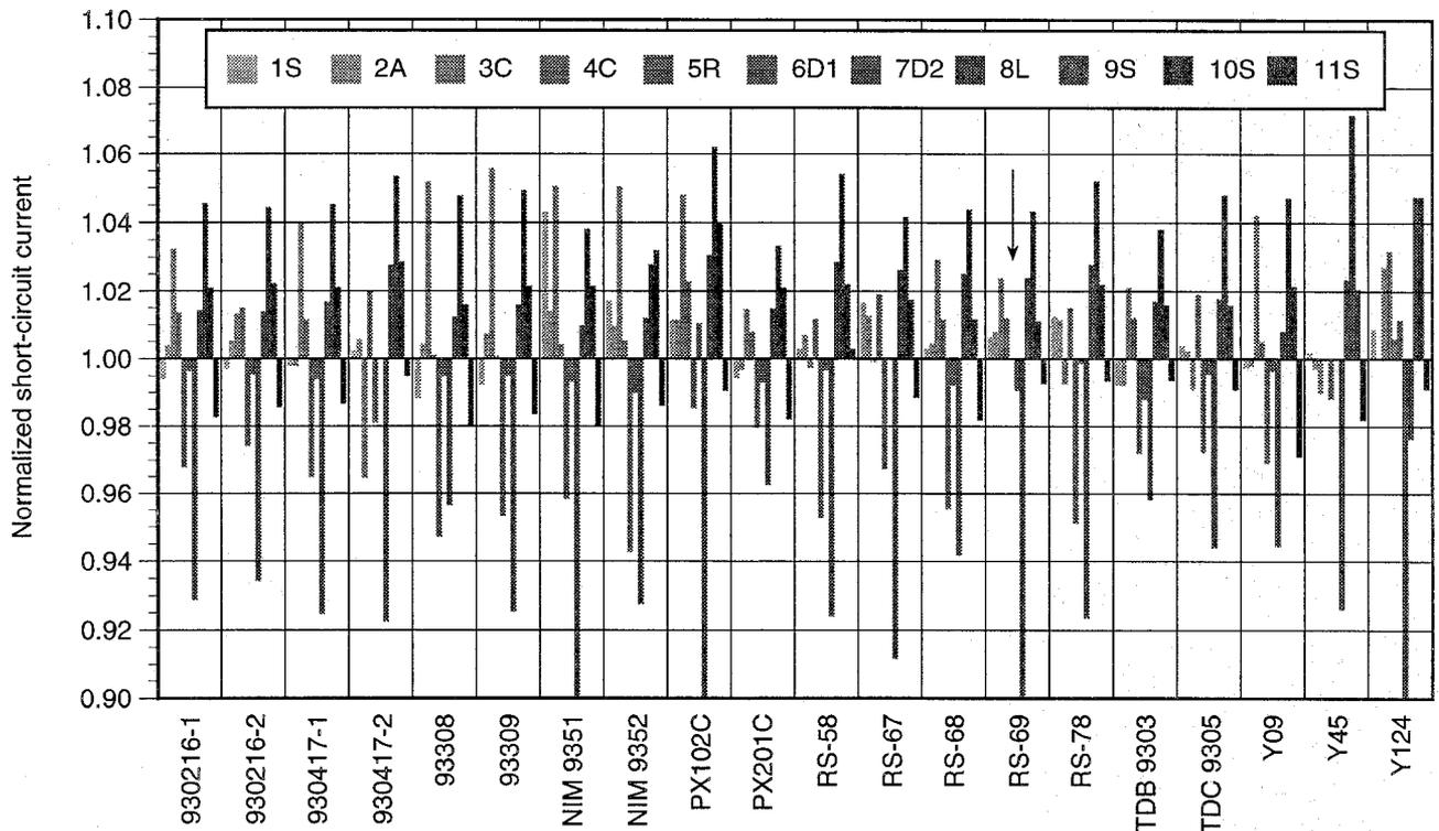
Fig. 1. Normalized 2x2 cm Si reference cell calibration results for the WPVS sample set. The  $2\sigma$  standard deviation is 7.3%. The laboratory designations indicate the order in which the samples were circulated and the calibration methods used (see text). The vertical arrow marks a missing data point.
