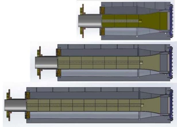
**Figure 5.** Family of Rancho S generators using 43 cm, 100 cm, or 144 cm detonation systems. Initial inductances are approximately 86 nH, 170 nH, and 225 nH respectively.
