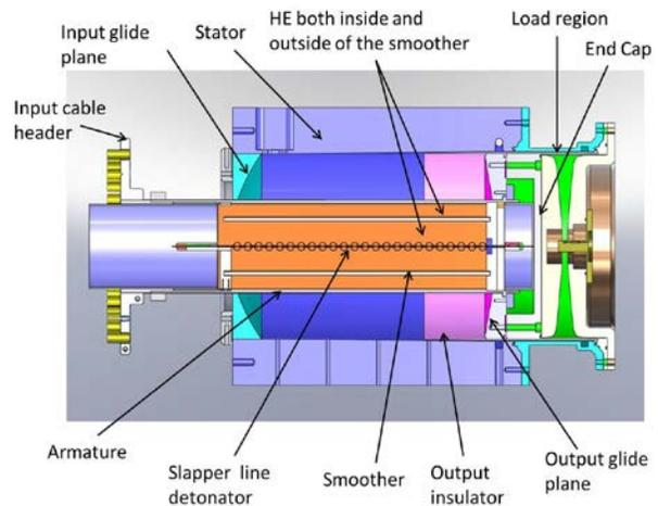
**Figure 1.** Baseline Ranchero configuration with 43 cm detonation system and an imploding liner load. For the minimum inductance load, the stator is connected to the output glide plane with a plate contoured to match the current joints shown here.
