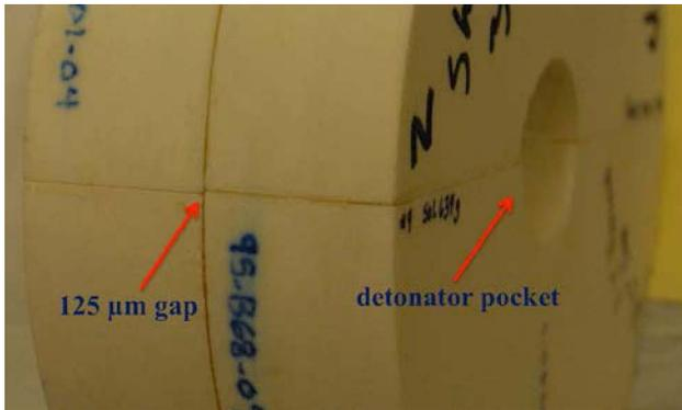
**Figure 7.** Armature charge with two 30 mm long 9501 half-cylinders glued together to create cylinders, and two of these glued together to make a 60 mm long cylinder. The detonator pockets were bored to different depths so that the middle of the 18 mm detonator spacing was offset by 3 mm from the glue joint. All glue joints were  $\sim 50 \mu\text{m}$  thick, but a machining error left an extra gap of 125  $\mu\text{m}$  at this compound joint, and it is seen to rupture in the dynamic record.
