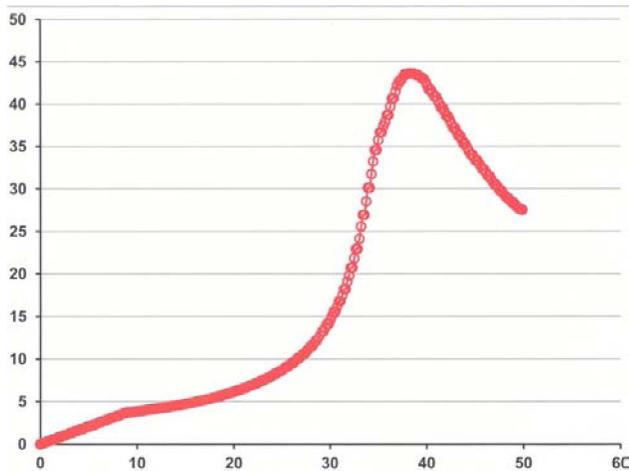
**Figure 9.** Current computed for 5 mm thick liner experiment. Seed current is provided by a 9.3  $\mu$ s ramp to 3.75 MA in this calculation.
