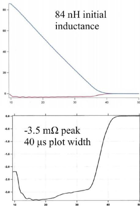
**Figure 4.** L and dL/dt for the FCG in Fig. 3. Operation time is from ~10 μs to ~40 μs.
