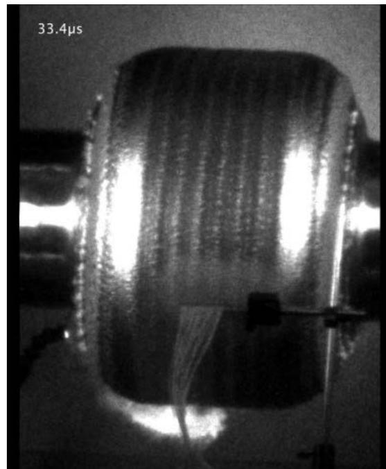
**Figure 6.** Framing camera record of armature expansion driven by 19.4 cm long 9501 initiated on 18 mm centers at the midplane of the HE cylinder. The 167 mm diameter, 6 mm thick annealed Al armature has expanded by a factor of two in this frame, and it is in good condition for flux compression.
