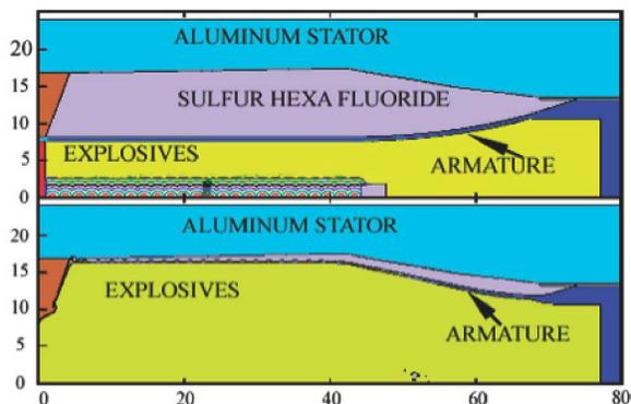
**Figure 3.** 2-D Hydrodynamic calculation of Ranchero S concept. There is no output glide plane in this design, and the armature is supported by full detonation pressure near the output. The first frame ( $t=0$ ) shows the initial contours and slapper initiation points, and the second frame ( $t=34.5\mu$ s) shows the contours as the armature approaches the stator. First armature motion is  $\sim$ 10  $\mu$ s. Inductance at first motion is  $\sim$ 86 nH, and at frame two is  $\sim$ 9 nH.
