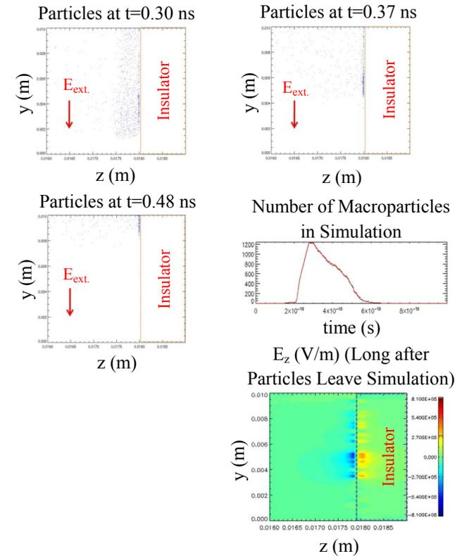
**Figure 7.** Cathode field emission takes place near the insulator surface. Secondary electrons with energies less than 0.4 eV are not emitted. The  $E_z$ -field indicates that there is a net gain of macroparticles from the insulator.
