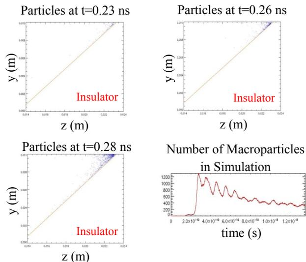
**Figure 9.** Insulator field emission takes place near the anode triple junction due to field enhancement. As the E-field increases electrons begin to emit further down the insulator towards the cathode.
