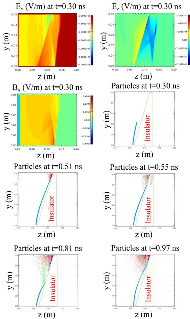
**Figure 10.** Flat top EM-pulse incident on insulator. The colored particles represent cathode field emission (light blue), anode secondary electrons (red) insulator secondary electrons (green) and insulator field emission (dark blue).
