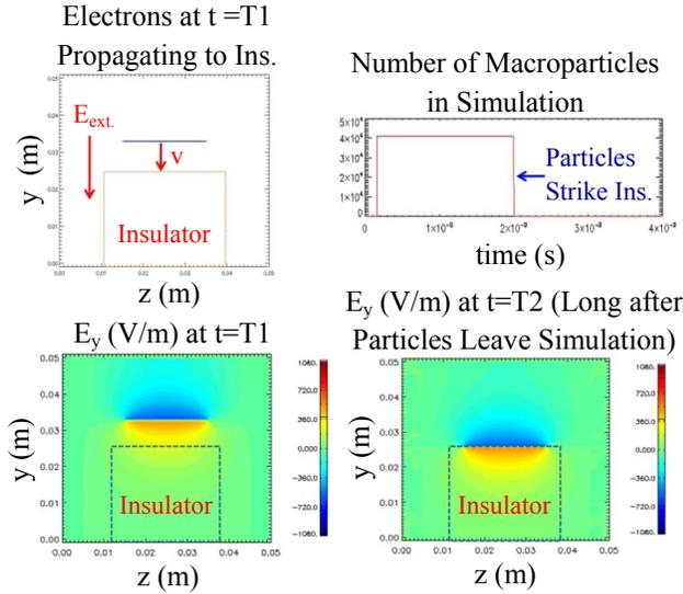
**Figure 4.** Illustration of insulator charge up when a beam of electrons is absorbed by an insulator, producing no secondary electrons. The  $E_y$ -field is shown with the external field subtracted out.
