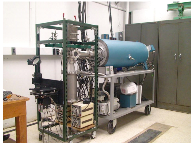
Figure 3. Photograph of the initial experimental setup with the 1 MV generator.
