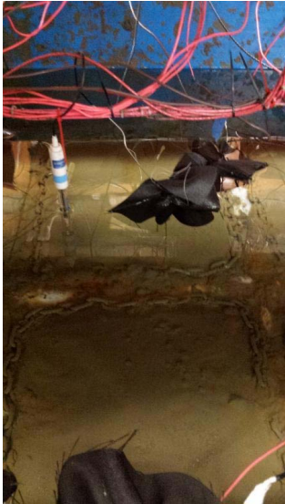
Fig. 3: 12in x 12in surface anodes with chain around the edges for sealing to sediment. The anodes have some sediment which settled on top of the BoPET however they can be distinguished by the chain around the edges.
