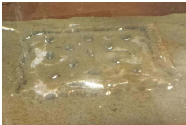
Fig. 2: Image of the surface anode after being placed on the sediment surface.
