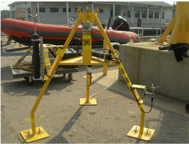
Figure 1. Bottom tripod with onboard instrumentation prior to deployment.
