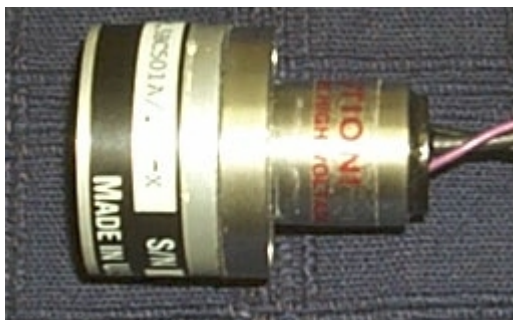
Fig. 8. Photo of the ½" x ½" liquid scintillator (BC501).
