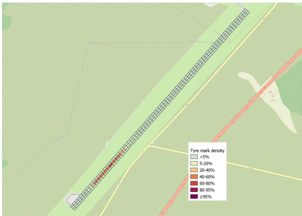
Figure 11 Whole runway surface area with visualized results for tire marks density
