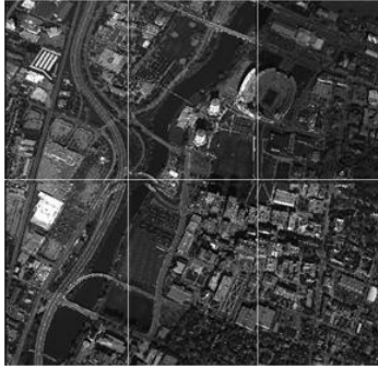
Figure 3. Example data from the CLIF LAIR sensor. The six different frames from one frame set are laid side-by-side to illustrate the need for an image mosaic.
