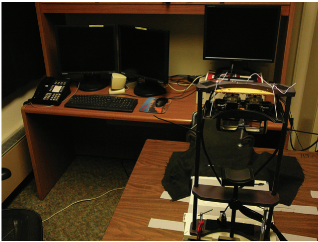
Figure 1: The experimental scene included the display eyepieces from our nVisorSR mounted on a chin rest (near right), a monitor to serve as the real world in the nVisorST's line of sight (far right), and two monitors to show the experimenter what image was being sent to the nVisorST (far left).
