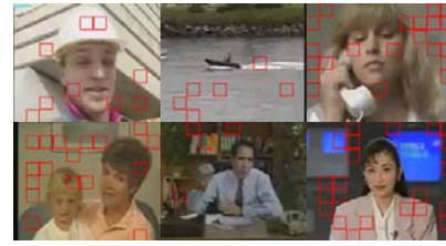
Fig. 8 Examples of inpainting mode MBs INPAINTING MODE RATIO UNDER DIFFERENT QP LEVELS
