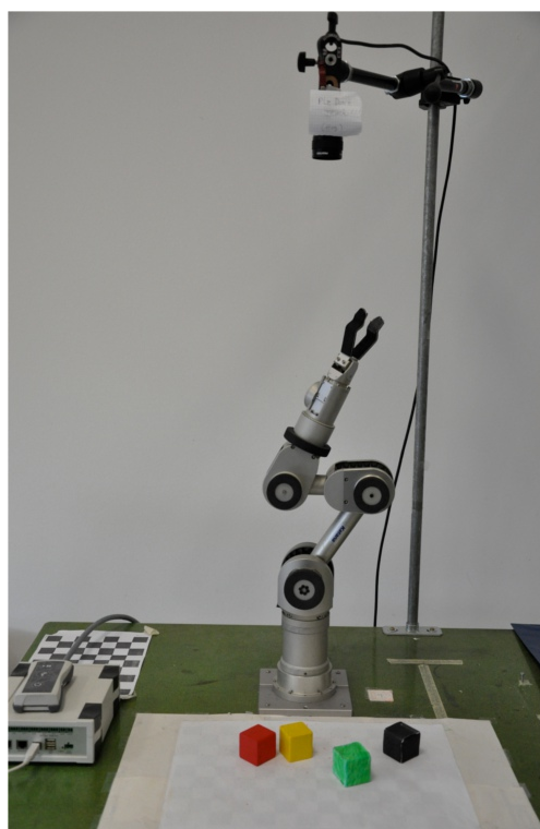
Fig. 1. The Katana robot arm in its block-world environment. It reaches for, grasps, and places blocks. The sensory input is an image from the overhead camera. There is a Markov Decision Process environment representation (discrete states and actions). Reinforcement learning updates a policy for action selection. The only reward is intrinsic: learning progress of a set of predictors (one for each state) that predict the outcome of that action. At any time, it prefers to try the state-action pairs that are associated with higher progress.
