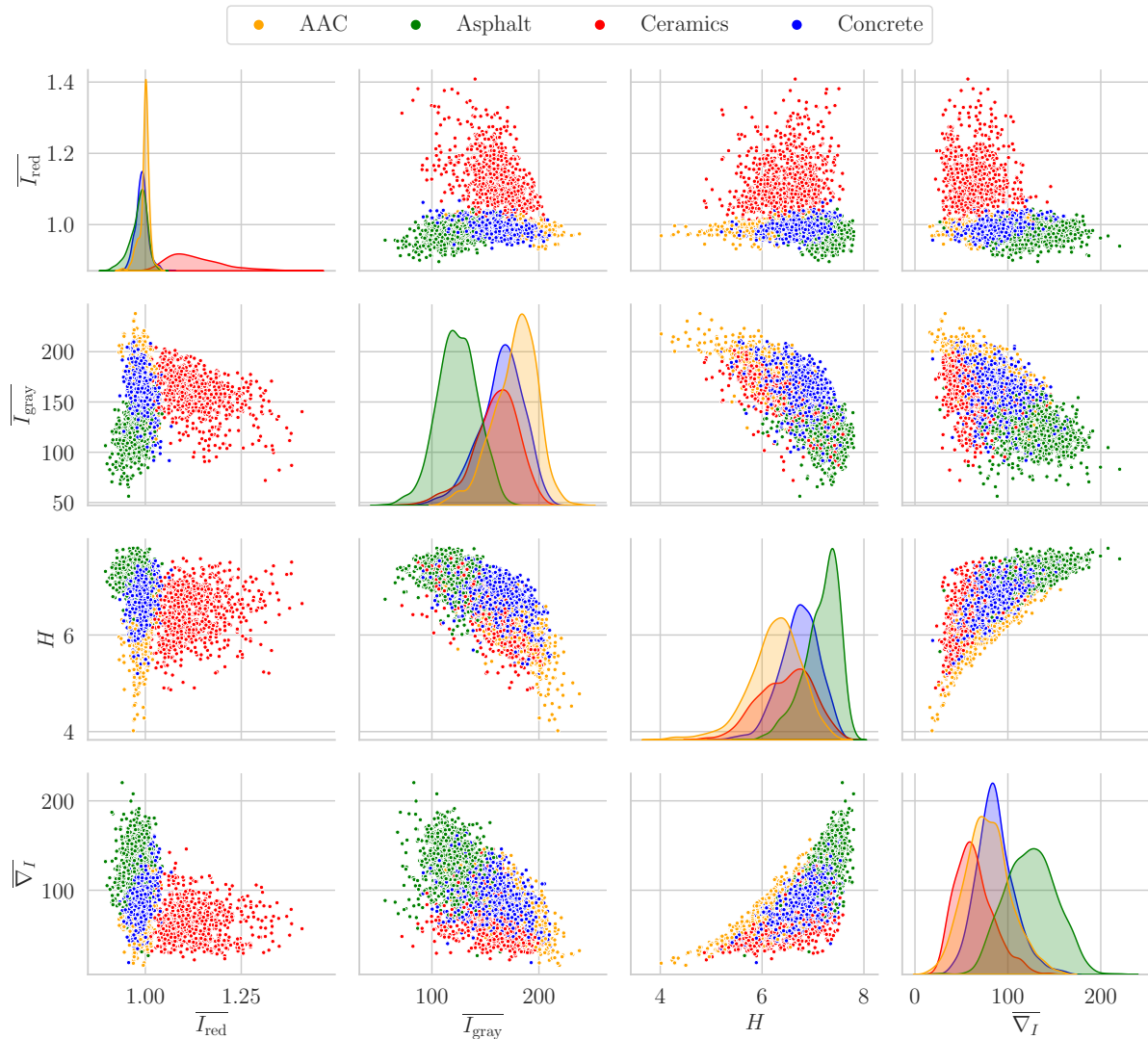
Figure 3.2: Visualization of the image subset characteristics for individual materials (classes) as pairwise scatter plots; marginal distributions of each feature for each class are plotted on the diagonal.
