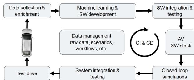
Figure 2: Data driven development of autonomous vehicles.
