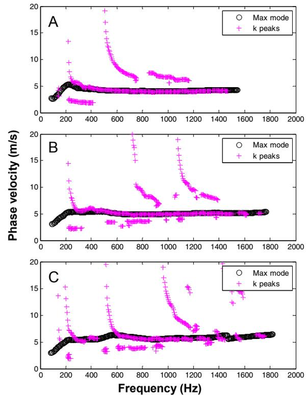
Fig. 5. Dispersion curves for different pressures calculated from the 2D FFT ( $k$ -space) plots. Panel A, B and C show the dispersion curves with different propagating modes for 10, 50 and 100 mmHg respectively. The solid circles show the prevalent mode for each frequency while the magenta crosses show the other modes propagating at each frequency.
