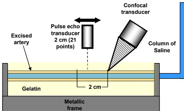
Fig. 1. Representation of the experimental set up for an excised pig carotid. Shear waves were generated using a confocal transducer and the propagation of the wave was measured with an ultrasound pulse echo system.
