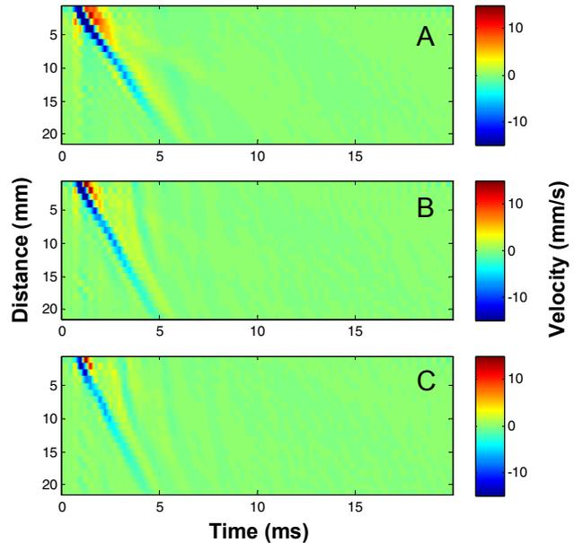
Fig. 3. Propagation of first impulse in the arterial wall at different pressures. Panel A represents the 10 mmHg, B, 50 mmHg and C, 100 mmHg.
