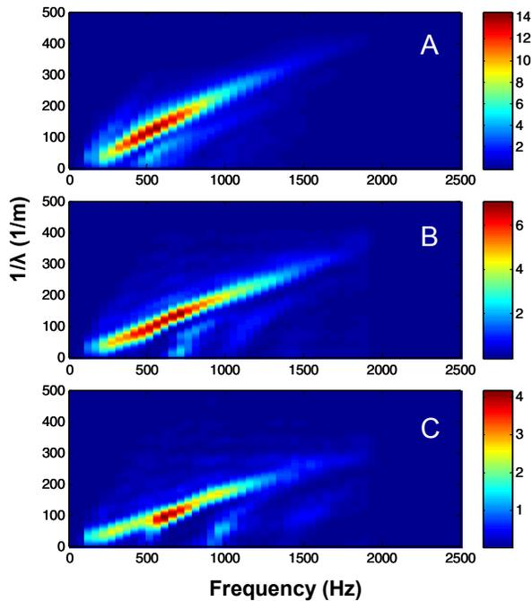
Fig4. Two dimension FFT representation of waves propagating on the arterial wall. Panels A, B and C show the results for 10, 50 and 100 mmHg respectively.
