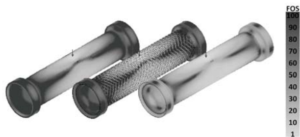
Fig. 5. An example of a stress analysis model for three cartridge designs. Left is the original design, center is a new design with a cross-helical reinforcing mesh, right is the same new design without the reinforcing mesh. Stresses are calculated as Von Mises stresses and reported a factor of safety (FOS) for reported values of molded polycarbonate.
