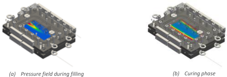
Figure 36: RTM process simulation of the composite plate POC 1 manufacturing.
