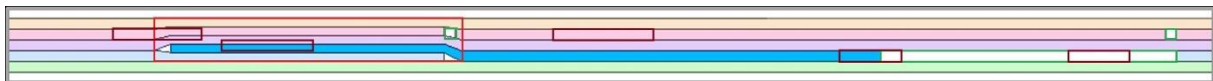
Figure 4.20 Example of areas of influence of an overlap (red) and gaps (green) some possible sets are highlighted in maroon, from left to right there would be two sets that belong to the overlap case, a set that has no defect and two sets that belong to the gap case.
