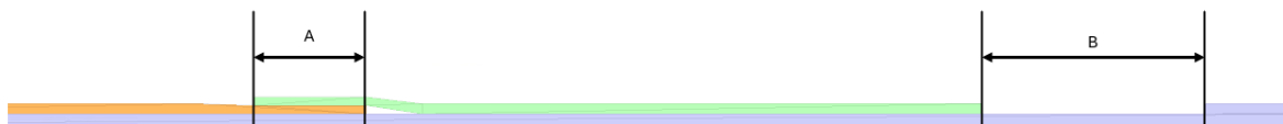
Figure 4.12 A represents the overlaid tow and B the gap generated because of the misplaced tow (overlap situation). Orange is the first tow allocated and green the second.
