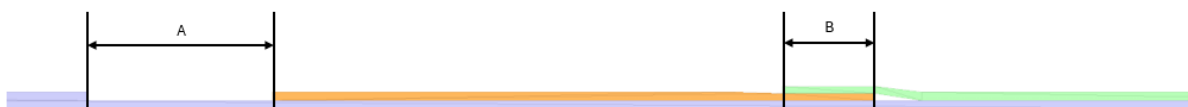
Figure 4.13 A represents the gap left by the AFP and B the consequence (gap situation). Orange is the first tow allocated and green the second.
