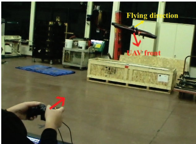
Fig. 2. Remote control of an UAV from the controller's perspective. In this example, pushing the joystick forward, the UAV will fly away from the user, instead of to the front of the UAV.
