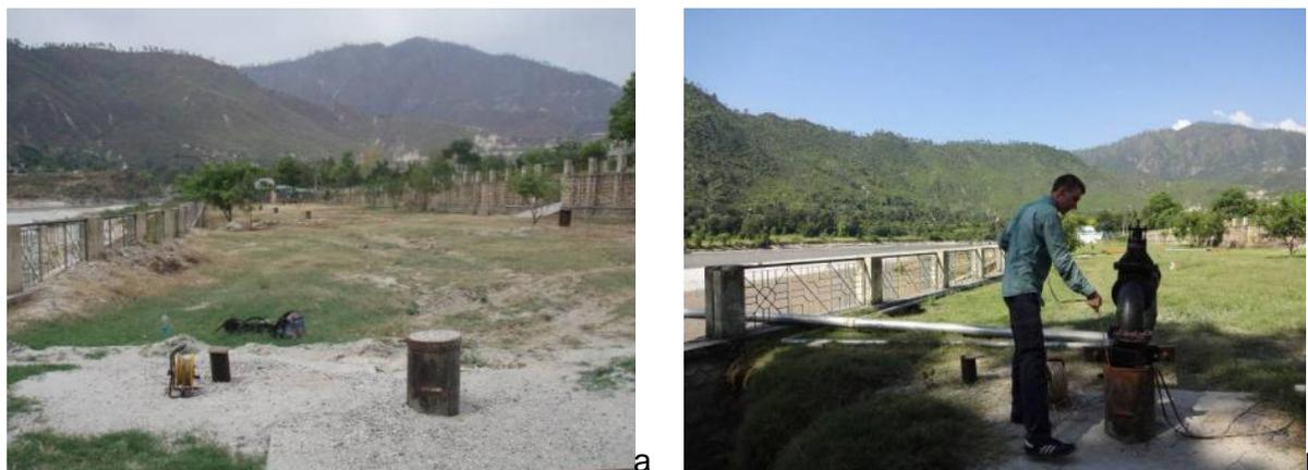
**Figure 16 (a) Monitoring well MW4 (left) constructed in Srinagar in between PW4 and the Alaknanda (Photo: K. Heinze, HTWD, May2012) (b) Pumping test and sampling being conducted on MW4 & PW4 (Photo: V.D.A. Nguyen, HTWD, September 2012)**
