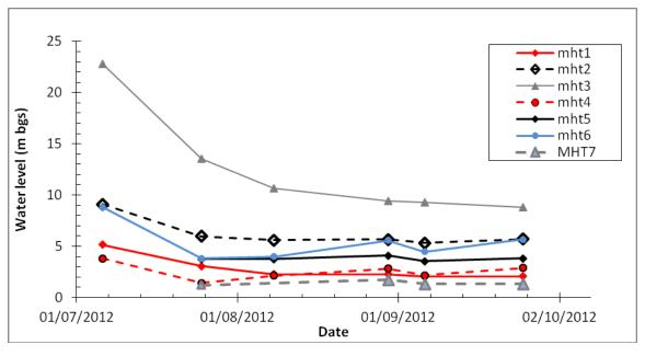
Figure 20: Water levels evolution in the piezometers
