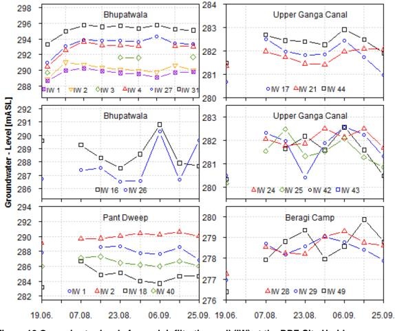
Figure 12 Groundwater-levels for each infiltration well (IW) at the RBF-Site Haridwar
