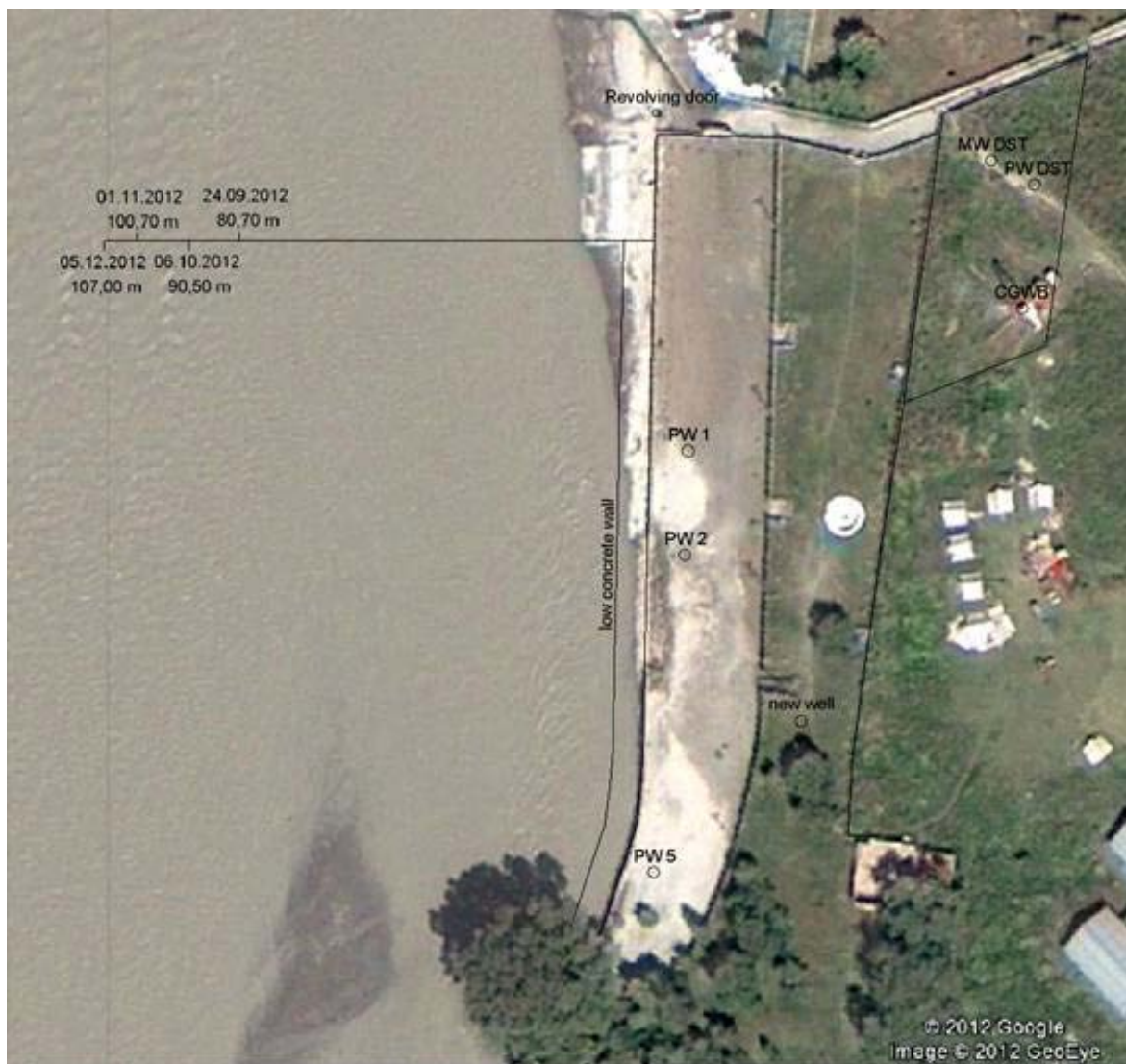
Figure 5-1 Retreat of the Alaknanda River's water line from September to November 2012 (Saph Pani, 2013)
