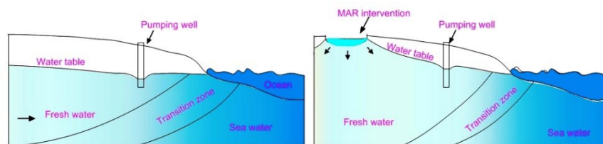
Fig. 4 Conceptual cross section showing (a) seawater intrusion due to overpumping and (b) MAR intervention for mitigation
