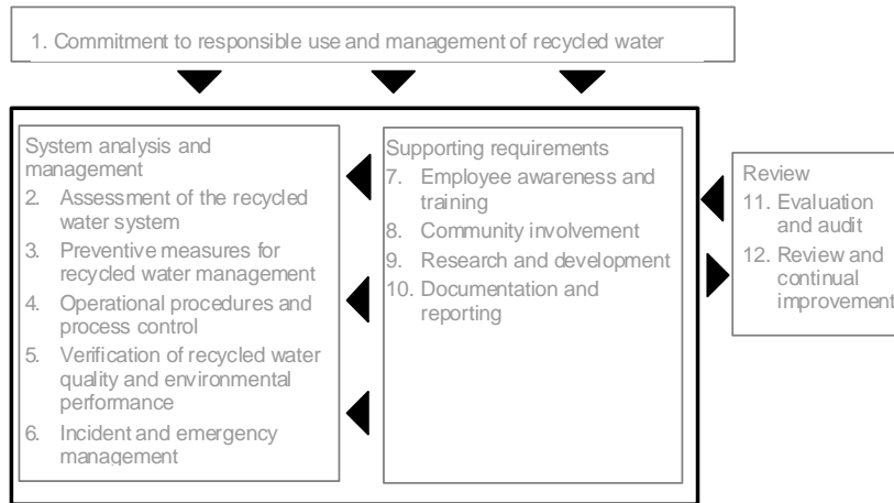
Fig.3. Elements of the framework for managing water quality and use (EPHC, 2008).
