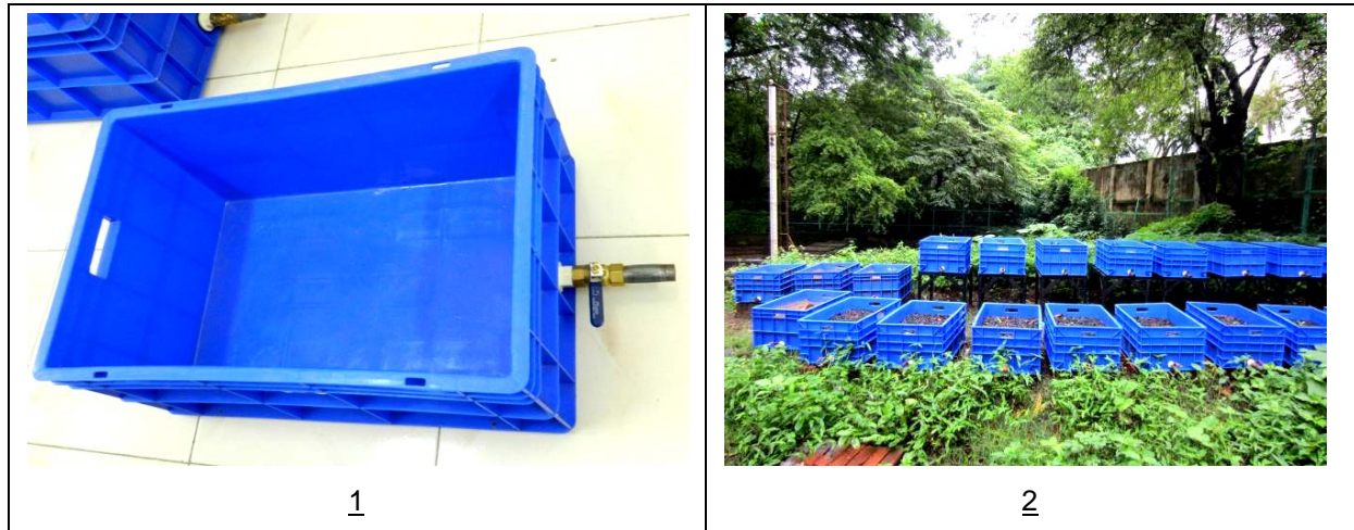
Plate 5.2: Crate used for experimental of constructed wetland reactors
