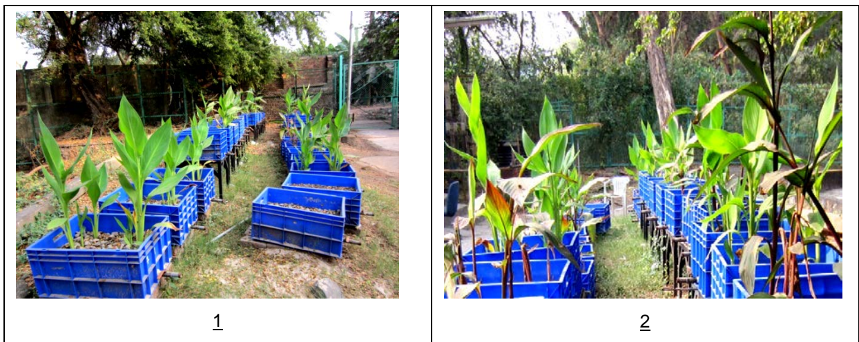
Plate 5.6: Experimental CW Reactors at sump well station (IIT Bombay)
