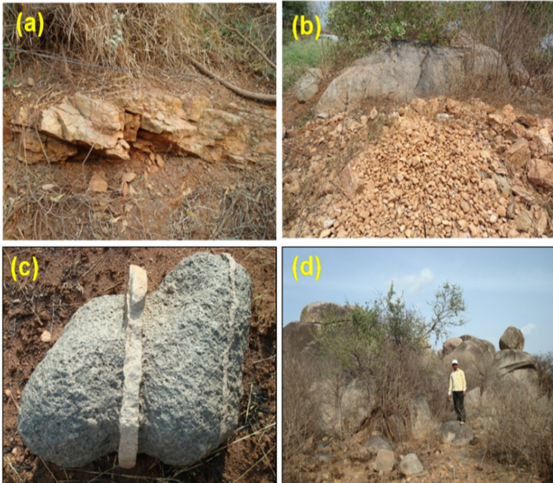
Figure 12 Field specimens showing the (a) weathered quartz pegmatite vein (b) weathered quartz with granite outcrops (c) quartz vein intrusion (d) outcrops of granite
