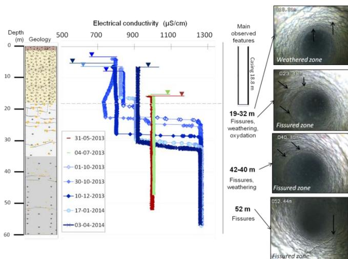
Figure 14. Geological log of MHT9 borehole; Electrical conductivity loggings evolution and fractures observed in borehole. Pre-monsoon campaign is shown in red, early stage of the monsoon (i.e. July 2013) is shown in green, and late stages of the monsoon and post-monsoon campaigns are shown in blue. Water level for each campaign is shown (triangles).
