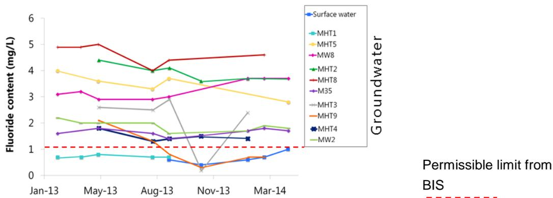
Figure 13. Evolution of fluoride concentration in the monitored boreholes surrounding the tank.
