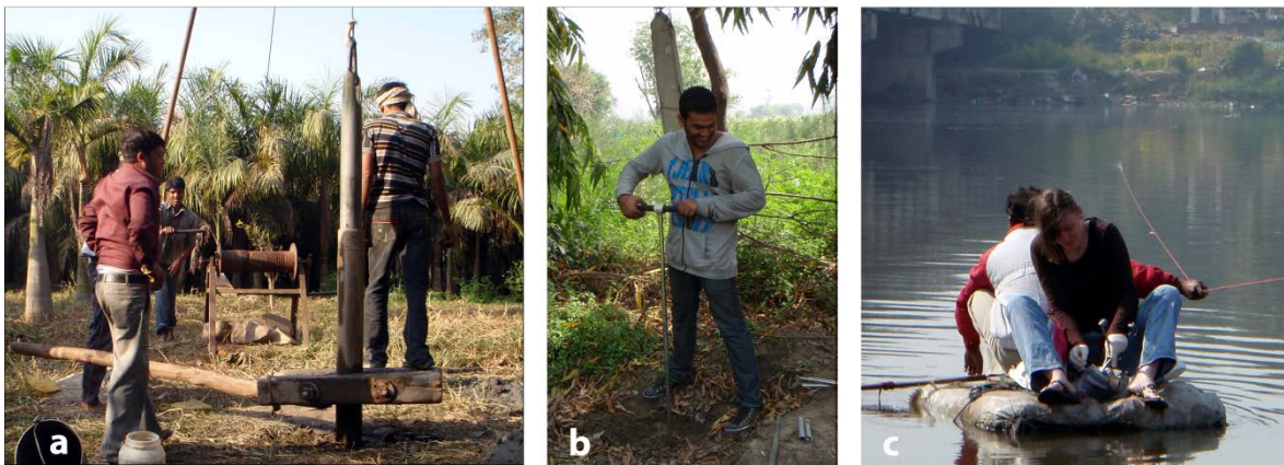
Figure 3 a. Manual auger drilling b. Shallow drilling with Eijkelkamp hand drilling device c. Sediment sampling of river bottom sediments
