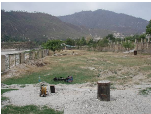
Figure 4-3 Monitoring well MW4 (left) constructed in between PW4 (right) and Alaknanda, Srinagar (Photo: HTWD, 2012)
