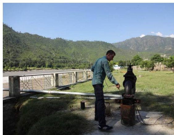
Figure 4-4 Pumping test and sampling being conducted on MW4 and PW4, Srinagar (Photo: V.D.A. Nguyen, HTWD, 2012)
