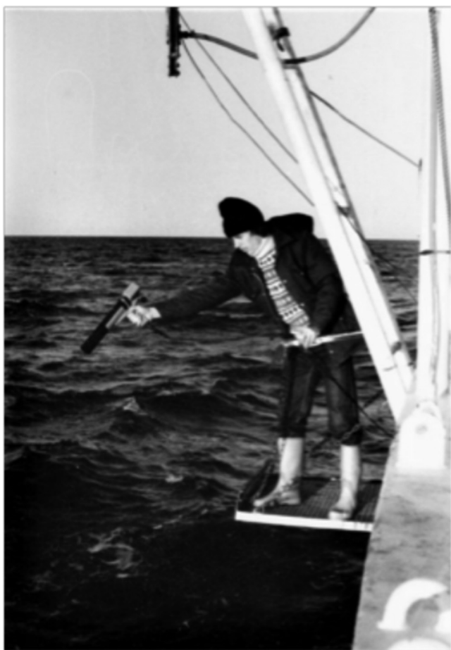
Figure 9. – Recording of a thermal profile using an expendable bathythermograph probe temperature recorder aboard the R/V Cryos in 1985 (Photo A. Forest).
