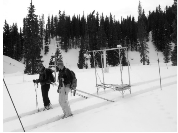
Figure 2. 2-10 GHz FMCW radar developed for alpine snow cover studies. This radar was used for crevasse detection.
