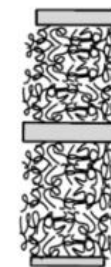
Meridional streaks from lamellae oriented in machine direction with different lateral sizes and thicknesses and with very high correlation lengths
