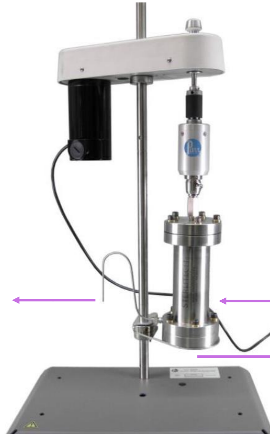
Pressurized filtration set-up
