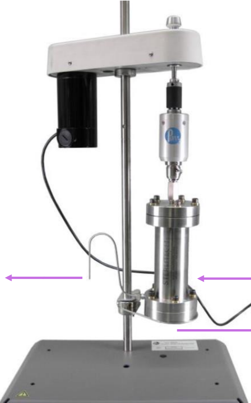
Pressurized filtration set-up Dead-end configuration
