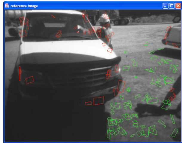
Figure 10. Captured image from one camera with ground and alarm areas identified.
