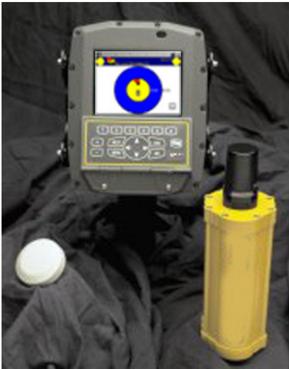
Figure 7. GPS system components. Left to right: GPS antenna, computer and display with integrated receiver, IP radio.
