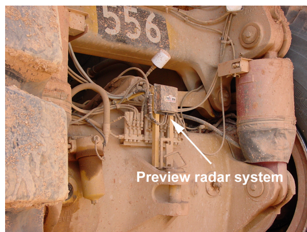
Figure 2. First version of Preview radar system mounted on Caterpillar 793B.
