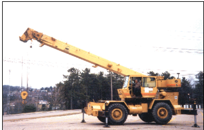
Fig. 3. 20 tonne (22 short ton) rough terrain crane used in experiments.
