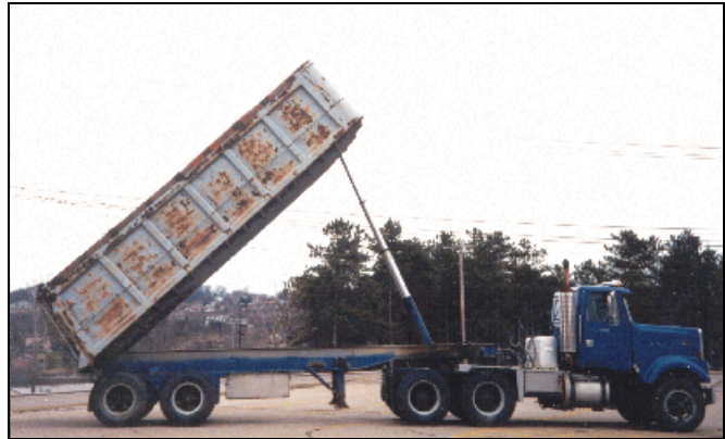
Fig. 2. 20.9 tonne (23 short ton) tractor-trailer dump truck used in experiments.
