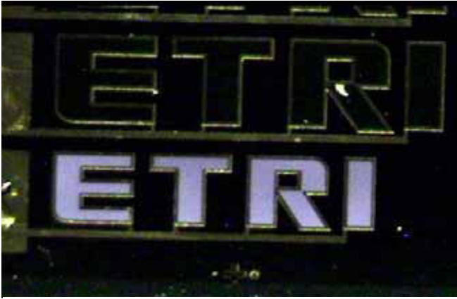
Fig. 4 Silicon-based visible light emitter showing the electroluminescence from a nc-Si active layer(lower ETRI Logo), which has high external quantum efficiency of 1.6%.
