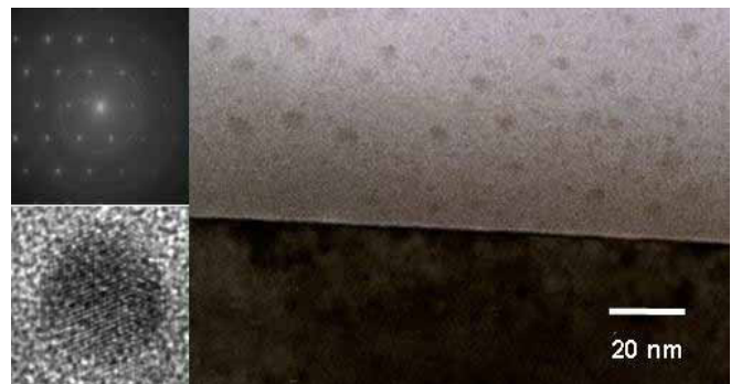
Fig. 1. Cross-sectional high-resolution transmission electron microscopic (HRTEM) images of nc-Si embedded in a silicon nitride film. The average size and the dot density of nc-Si was 4.6 nm and 6.0 \times 10^{11}/\text{cm}^2 , respectively. The insets are the crystal image and the transmission electron diffraction pattern, showing silicon dot is crystalline.
