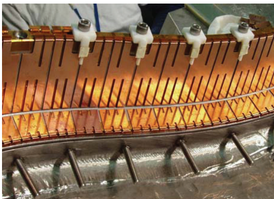
Figure No. 9- Copper Chill Plates in Position
