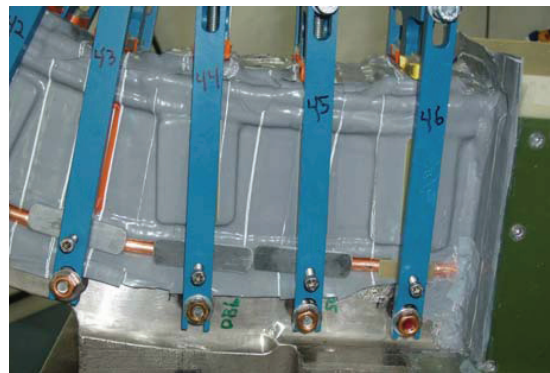
Figure No. 7- “Bag Mold” Under Vacuum
