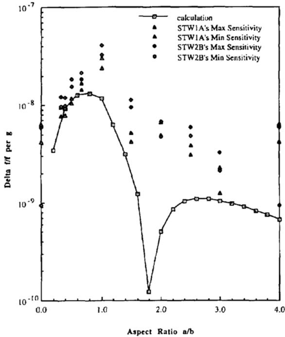
Figure 5. Comparison of measured and calculated STW normal acceleration sensitivity.
