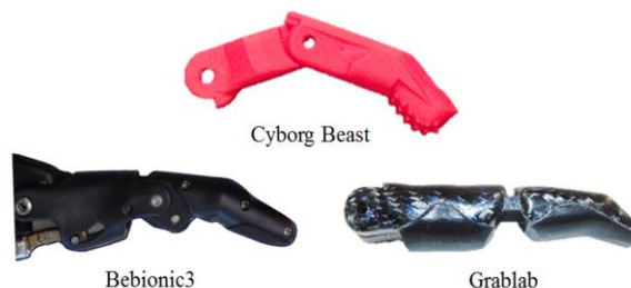
Figure 1. Fingers from the 3D Printed Cyborg Beast hand [1], the Bebionic v3 [3], and Composite prosthetic finger created using additive manufacturing molding techniques.
