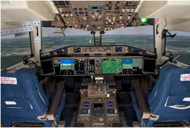
Figure 1. Research Flight Deck Simulator with HUD and Head-down Instrument Panel
