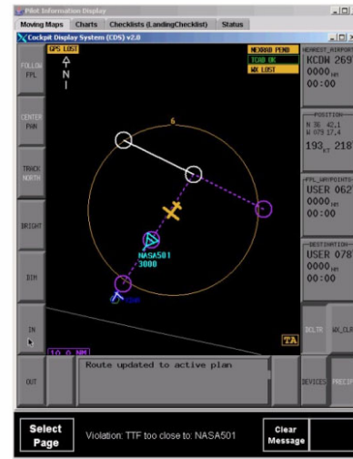
Figure 12. The ‘Cockpit Associate’ Aids the Pilot in Flying Safely and Proficiently by Conducting Situation Assessments, and Providing Recommendations and Advisories
