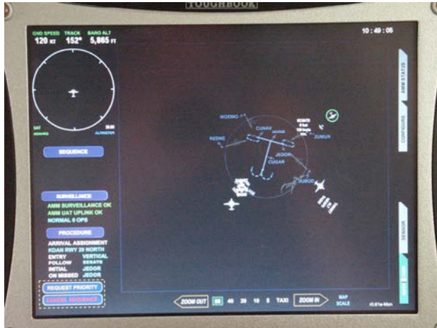
Figure 11. The Electronic Flight Bag Provides the Pilot HVO Functionality and Flight Information at the Danville SATS SCA
