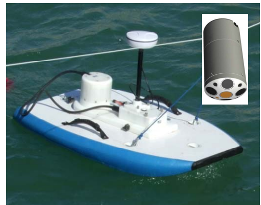
Fig. 9. Photograph of the RiverSurveyor M9 (inset) deployed in the small SonTek hydroboard.
