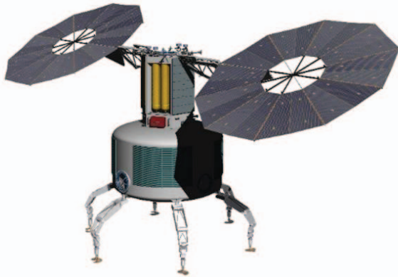
Figure 2. Illustration of the mobile habitat with the chemical/solar electric propulsion delivery vehicle attached. The habitat is equipped with legs capable of hexapodal translation across Phobos surface.
