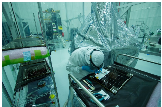
Figure 15: Cell Repair at the Launch Facility
