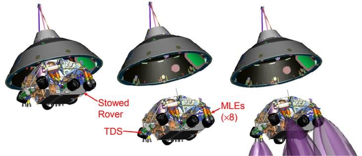
**Figure 4 – Backshell Separation and Freefall Sequence**
