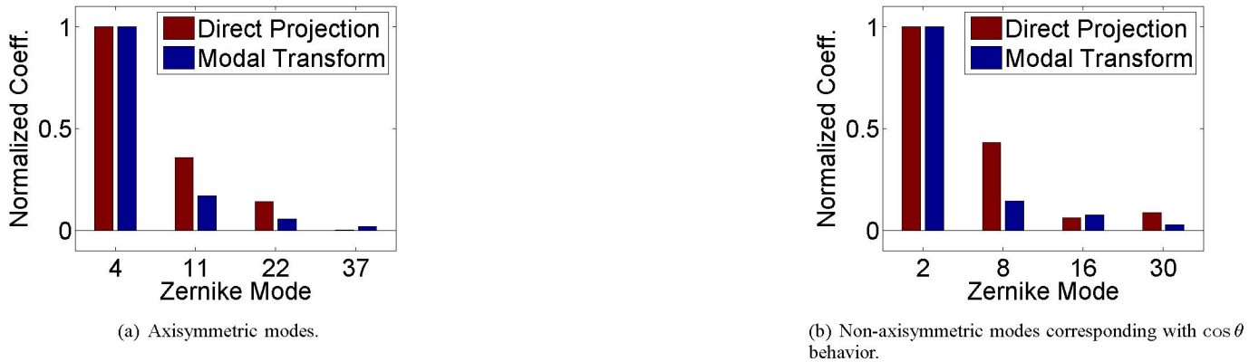
Fig. 12. Comparison of Zernike mode coefficients for actuated surface for matrix modal transformation methodology versus direct projection methods as described in text. The desired Zernike modes were 2 and 4. Values of coefficients for other modes represent undesired surface deflection.
