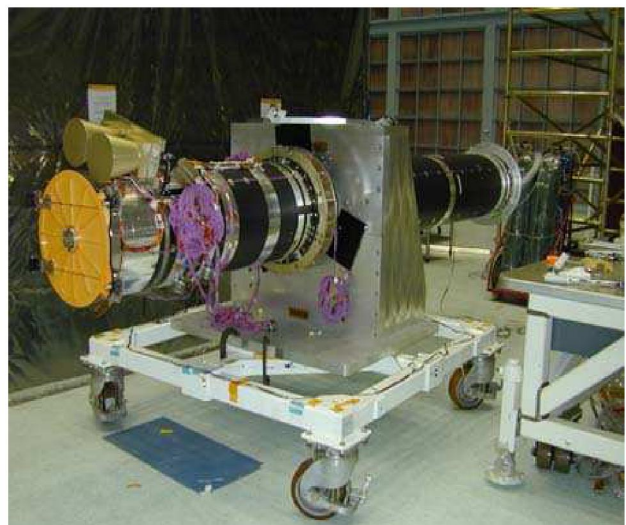
Figure 1.0(c): The XRT instrument shown during I&T at the GSFC. Note the Star Tracker simulators attached to the forward tube.
