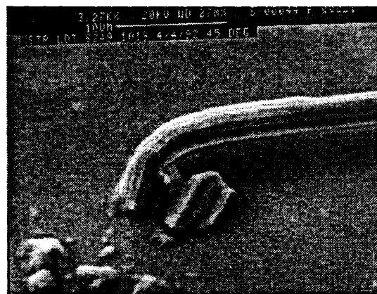
Fig 2. Primary whisker growth is associated with eruptions of tin nodules, and often whiskers appear to grow out of these nodules. Note the striations along the body of the whisker. (SEM photo courtesy of the Aerospace Corporation)
