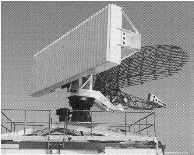
Fig. 2. Photo of mechanically rotating back-to-back experimental Senrad antennas; one is a conventional parabolic reflector, the other is a low-sidelobe planar array.
